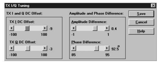
TX I/Q Tuning has following items: Tune TX I DC Offset scroll bar (ALT+I): The DC Offset is shown as percents (%) from the  $\pm$  maximum value. 0% means that there is no DC. The value range is -100%...100%. The value is rounded to the nearest integer value.
